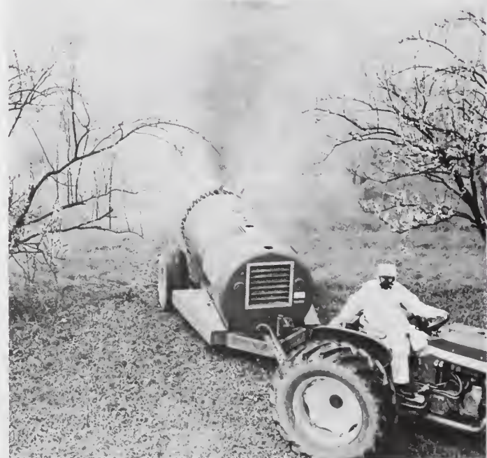
Figure 12: Air-concentrate mist blower used to spray bush fruits, grapes, and compact high-density tree fruits.
